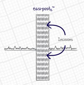
This process allows the preservative treatment to permeate the timber to a deeper level, achieve the Use Class 4 requirements and therefore a longer lifespan of the post is achieved.
